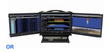
Real-Time Outdoor Spectrum Analyzer (IP65 rated) with fully featured PC and Drone Detection Software
